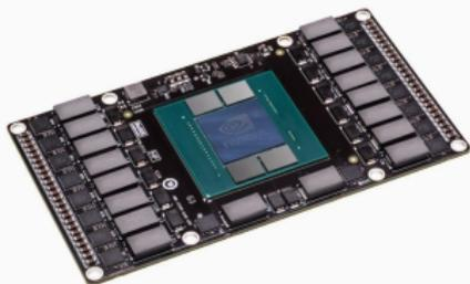
**NVIDIA Tesla V100:** World's first GPU to break the 100 teraflops barrier of deep learning performance. New feature: 640 tensor cores. Relatively cheap ( $\approx$  \$8,000). Released June 2017.
